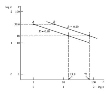
The R = 0.20 locus is above and parallel to the R = 0.90 locus. For the two-parameter Weibull distribution,  $x_0 = 0$  and points A and B are related by [see Eq. (20-25)]:
